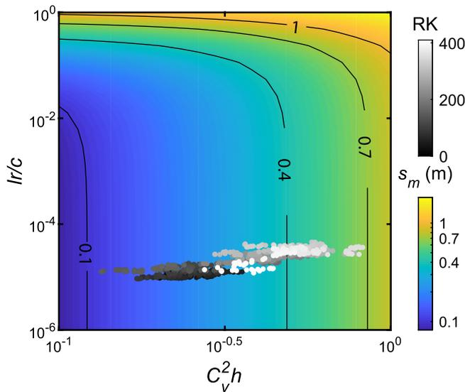
**Figure 3. Numerical model of cross-set thickness ( $s_m$ ; contours) for various rates of aggradation and distributions of dune size. Abscissa ( $C_v^2 h$ ) and ordinate ( $lr/c$ ) axes correspond to second and first terms on right side of Equation 1, respectively. Gray-scale color-coded dots are model results of cross-bed thickness for Mississippi River (MR). RK—river kilometer.**
