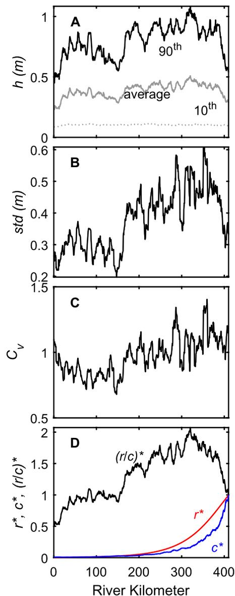
**Figure 2. (A) Spatial variation in dune height ( $h$ ). (B) Standard deviation in dune height ( $std$ ). (C) Coefficient of variation in dune height ( $C_v$ ). (D) Backwater morphodynamic model of lower Mississippi River (MR), showing spatial variations in key modeling parameters (normalized by value of each parameter at river kilometer 410), including normalized aggradation rate ( $r^*$ ), dune celerity ( $c^*$ ), and ratio of ( $r/c$ )<sup>\*</sup>.**
