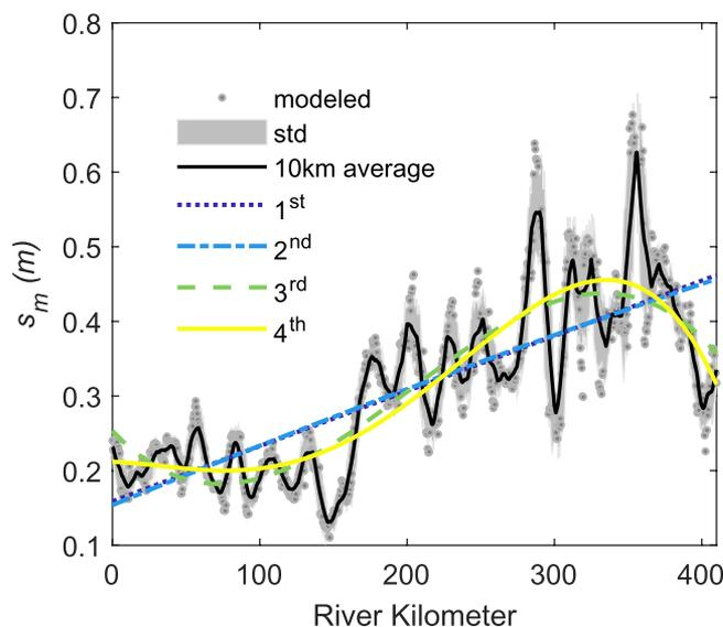
**Figure 4. Spatial trend of modeled cross-set thickness,  $s_m$ , for Mississippi River (MR). Black solid line is 10 km average in cross-set thickness, with associated one standard deviation (std) marked in gray. Dark blue, light blue, green, and yellow lines represent linear, quadratic, cubic, and fourth-order polynomial regression functions fit to cross-set thickness, respectively.**
